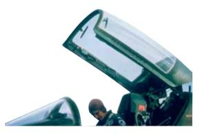
Made from high optical quality Lexan resin, Lexan Margard MR5E sheet is UV- and mar-resistant, and virtually unbreakable. It is an excellent option for windscreens and glazing used in recreational and off-road vehicles.
