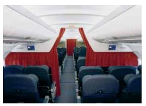
Adder cabin divider SABIC Innovative Plastics provided parts made from Ultem\* 1668 sheet to Airbus aircraft for the development of Adder cabin dividers.
