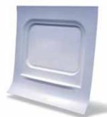
Train window mask from Azdel<sup>†</sup> Rail-Lite composite used on the Long Island Railroad, New York. Azdel Rail-Lite composite, a breakthrough technology from Azdel, Inc., and SABIC Innovative Plastics, is a new Iow-pressure, thermoformable, lightweight composite sheet that exhibits excellent flame, smoke, toxicity, and heatrelease performance in large semi-structural train panels.
